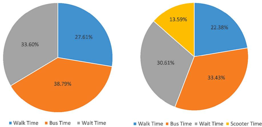
Fig. 3. Travel time composition without (left) and with (right) the micromobility service.
