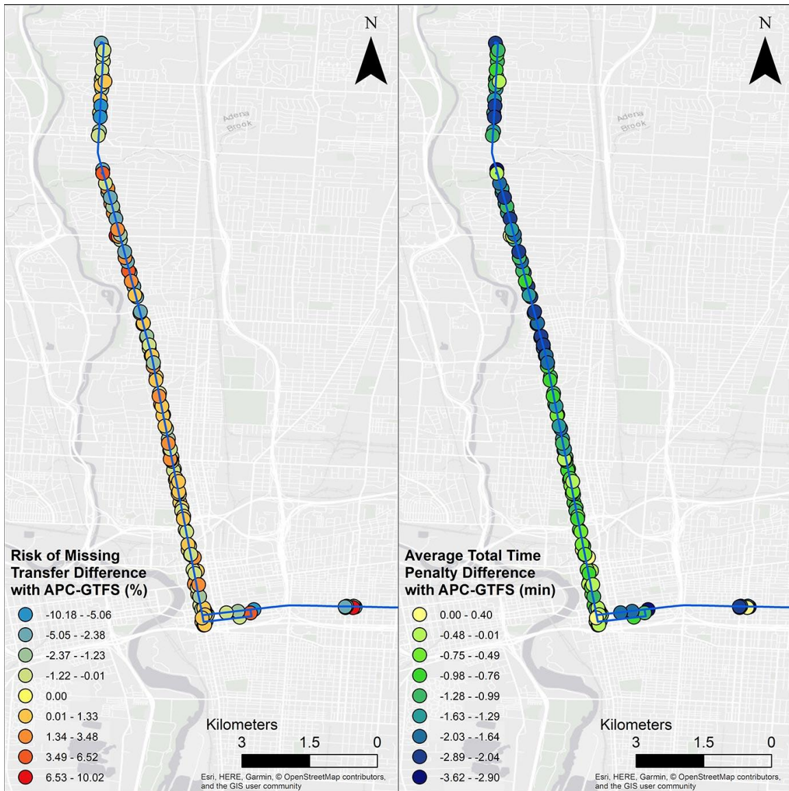
Figure 7: RoMT and ATTP difference after simulated implementation of a dedicated bus lane.
